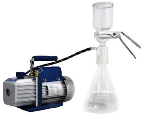
Figure 1. Membrane filtration system
