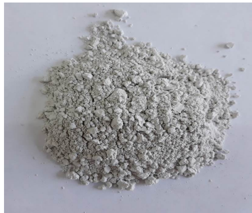
Figure 5. The fraction after magnetic enrichment, crushed in a porcelain ball mill to the state of powder (from the fraction d = -1 mm).
